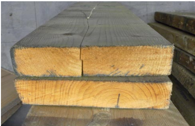
Cut ends need to be coated with preservative
