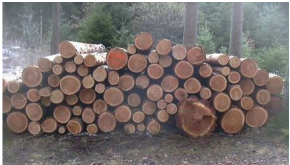
Figure 2: Freshly cut logs showing the pale sapwood rim and the darker heartwood centre
